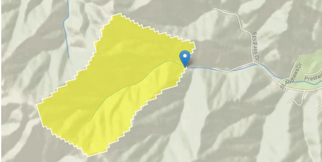
Figure 2. Bridge 2 watershed area delineated in Streamstats.
